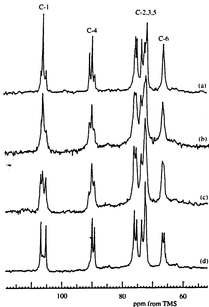
Figure 12 50 MHz CP/MAS ^{13}\text{C} NMR spectra of Valonia cellulose annealed at different temperatures in 0.1 N NaOH solution: (a) original; (b) 220 °C; (c) 240 °C; (d) 260 °C. 87
